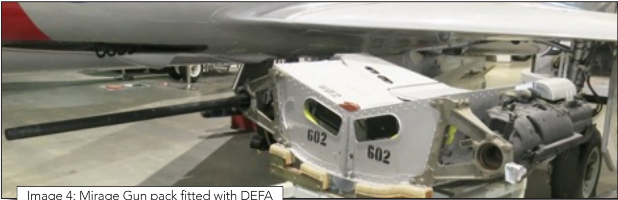
Image 4: Mirage Gun pack fitted with DEFA Cannon, Fighter World Museum at RAAF Williamtown. Source: Author.
