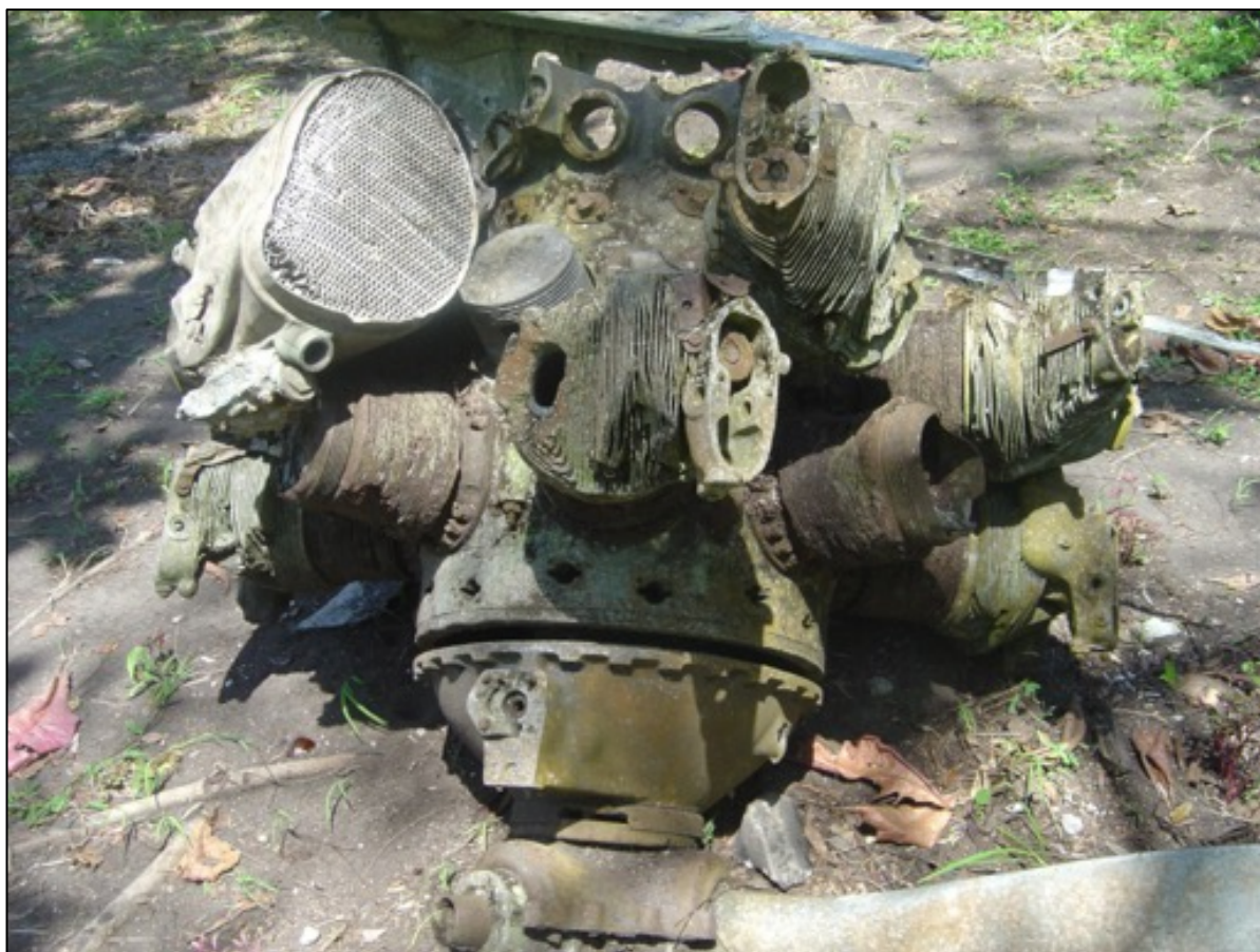
Figure 2: 14-cylinder Wright R-2600 Twin Cyclone radial engine located at the wreck site. Source: J.R. Taylan/Pacific Wrecks, 2005.
