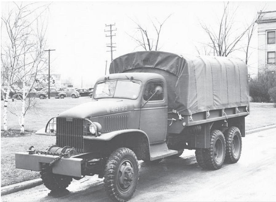
Figure 1: A CCKW-353 2.5 ton 6x6 truck fitted with winch. Source: Wikipedia.
