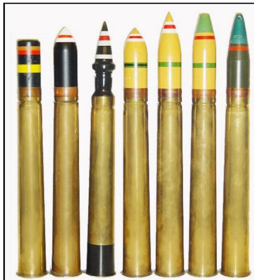
Various 2 pr complete munitions (L to R): Prac Flat Head, AP/T, APCNR/T, HE Mk I, HE, HE/T Mk XI, HE/T Mk VII
